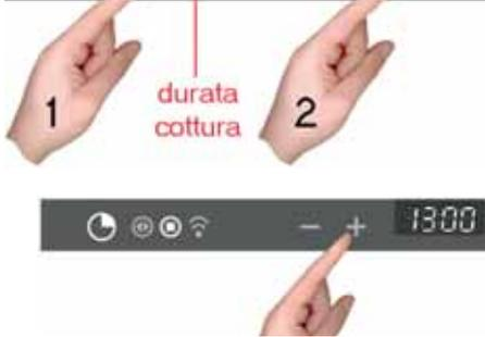
Now, set the end-of-cooking time: the control normally adds the cooking time to the current time, so it proposes an end-of-cooking time, which in our case would be 10:30 (8:30+2:00).
