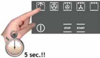
To disable the demonstration mode, touch the light symbol for five seconds: the oven will go to normal operation and be ready for turning on. Now you can set the time but it is not necessary for turning on the oven.
