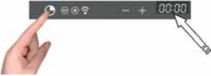
The separator dots flash to indicate that you can set the time.
