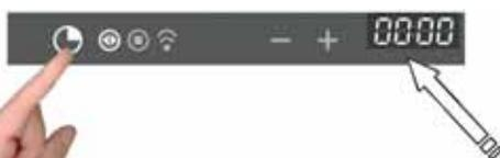
Touch the timer symbol once and the relative symbol will light up. Plus, the clock display will replace the current time.
