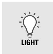
This pad turns the **night light** in the dispenser on and off. The light also comes on when the dispenser pad/cradle is pressed. If this light burns out, it should be replaced with a 6 watt 12V maximum bulb.
