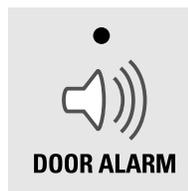
To set the alarm, press this pad until the indicator light comes on. This alarm will sound if either door is open for more than 3 minutes. The light goes out and the beeping stops when you close the door.
