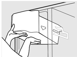
② Lift and pull forward again to remove the bin.
