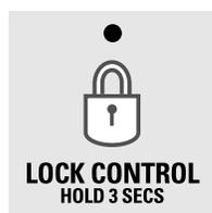
Press the **LOCK CONTROL** pad for 3 seconds to lock the dispenser and control panel. To unlock, press and hold the pad again for 3 seconds.
