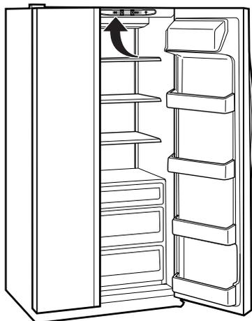
The temperature controls are preset in the factory at **5** for both the refrigerator and freezer compartments. Allow 24 hours for the temperature to stabilize to the preset settings.
