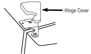
**NOTE:** DO NOT use a screwdriver to remove the cover. BE CAREFUL not to break the rear retaining tab on the hinge cover. Remove the hinges using a Torx T-20.
