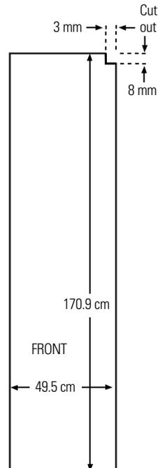
The areas at the top of the panels need to be cut out of the panels.
