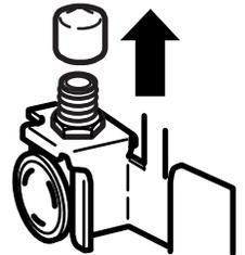
Place the compression nut and ferrule (sleeve) onto the end of the tubing as shown.
