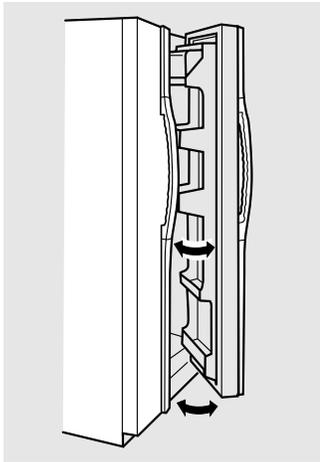
When the door is only partially open it will automatically close.
