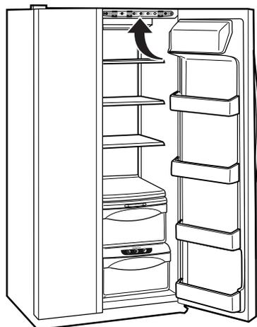
The temperature controls are preset in the factory at **3°C** for the refrigerator compartment and **-18°C** for the freezer compartment. Allow 24 hours for the temperature to stabilize to the preset recommended settings.
