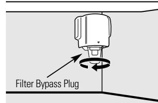
You must use the filter bypass plug when a replacement filter cartridge is not available. The dispenser and the icemaker will not operate without the filter or filter bypass plug.
