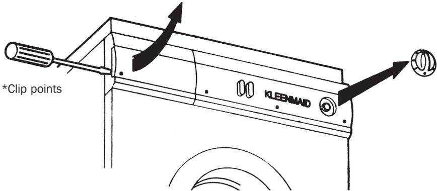
Hook the top edge of the replacement panel into the dryer, and clip in the bottom edge at the four points. Ensure that the three location pegs are engaged. Replace the timer knob ensuring that its flat is aligned with the flat on the timer shaft.
