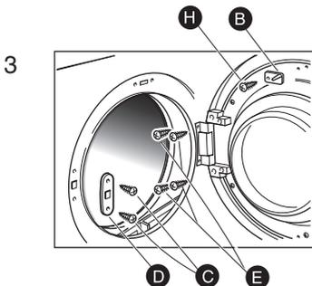
Refit latch plate (D) with screws (C). Remove screw (H) at top of door and refit switch strike (B) as shown. Fit door to hinge blocks and secure with screws (E).
