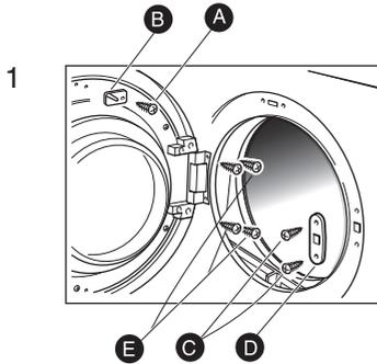
Open the door. Undo screw (A) remove switch strike (B) and replace screw. Remove screws (C) and latch plate (D). Remove hinge block screws (E). Remove door from hinge blocks.
