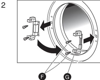
Remove hinge screws (F) and hinge (G) and refit to opposite side as shown.
