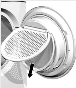
**⚠ If the filter is not regularly cleaned, the airflow is obstructed, which causes longer drying time and danger of overheating.**
