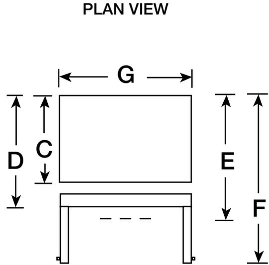
The minimum clearance behind the refrigerator is 25mm. This allows for the water pipe to connect to the refrigerator. Please ensure the water and tap electrical point are located in an adjacent cupboard (within 1 metre of either side of the unit), or above (within 100mm of the height of the refrigerator) rather than behind the refrigerator. Additional clearance will be required if the utilities are located directly behind the refrigerator.
