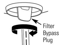
The icemaker and dispenser will not operate without the filter or filter bypass plug installed.
