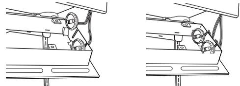
9. Insert the tabs on the back of the light housing in the slots on the back wall. Raise the light housing into position and secure with the four screws.
