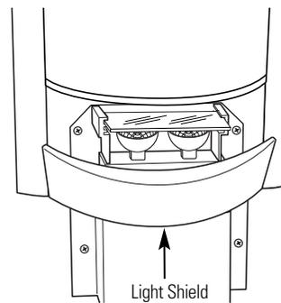
**WARNING:** The light shield must be replaced or the heat from the bulb could damage the refrigerator.
