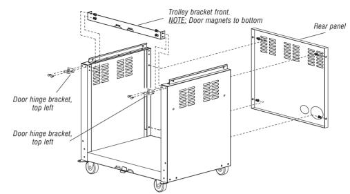
(5) Insert the bottom door hinge pin into the lower door hinge bracket holes. Depress the spring loaded top door hinge pin and line up with the top hinge bracket holes, and release the pin. Attach door handles.
