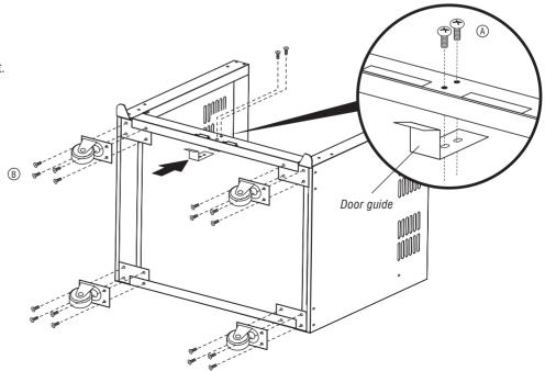
4 Attach the trolley bracket front and rear panel.
