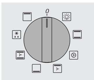
Turn the selector knob clockwise to the position corresponding to the function required (see cooking guide). The cooling fan will operate and the light will come on.
