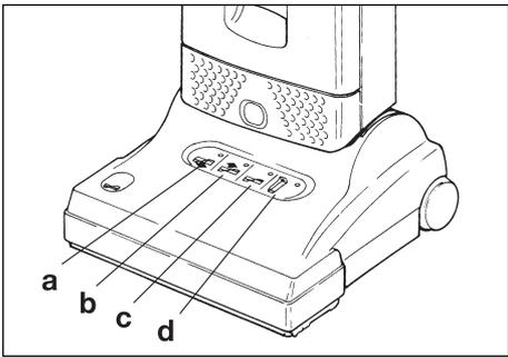
The machine has an information display on the power head with four lights to monitor the automatic functions.
