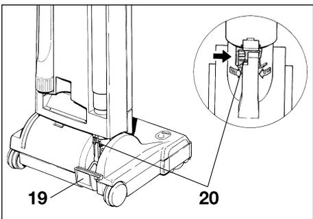
To release the machine from the upright position, press the foot pedal (19) down. With the orange slider (20) an intermediate stop position can be added to lift the brush over obstacles. Then to lower the machine to the horizontal position, press the foot pedal again.
