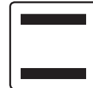
Traditional cooking: upper and lower heating elements Pizza and Bread
